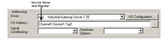
The I/O address for the driver has the following format: Channel\_Name.Device\_Name.Tag\_Name
