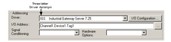
Note: For Database Manager to recognize the acronym entered, it must appear in the SCU's Configured I/O Driver list box.
